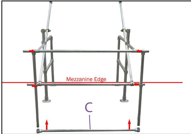
**12.** On opposite end to mezzanine edge insert part (C) horizontal tube by sliding tube 4" up the vertical posts. Tighten using 1/4" hex key.
