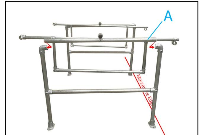
5. Take part (A) with hinge arm and mount wide size 8 (1.90" dia) tube to frame with gate rail on inner side. Repeat this step for other frame. NB. Slight loosening of the frame may be required to allow the horizontal to be inserted into the frame.
