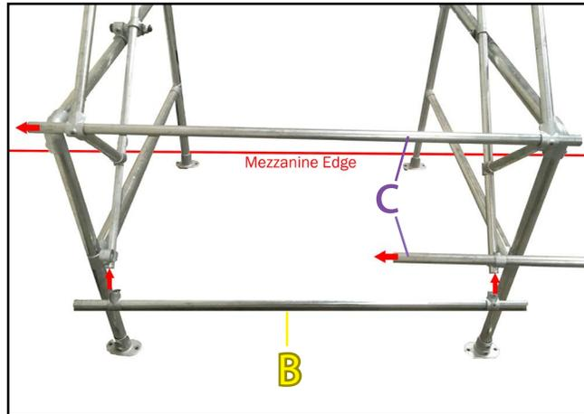
**7.** On opposite end to mezzanine edge add 2no. part (C) horizontal tubes to upper and lower cantilever tubes. Then add part (B) onto ends of lower cantilever tubes. Tighten using 1/4" hex key.
