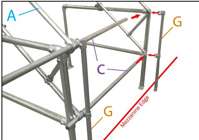
**6.** Rotate cantilever part (A) so this is as above. Add 2no. part (C) horizontal tubes on mezzanine edge end and add part (G) upright tubes as above onto parts (C) during the process. Tighten using 1/4" hex key.
