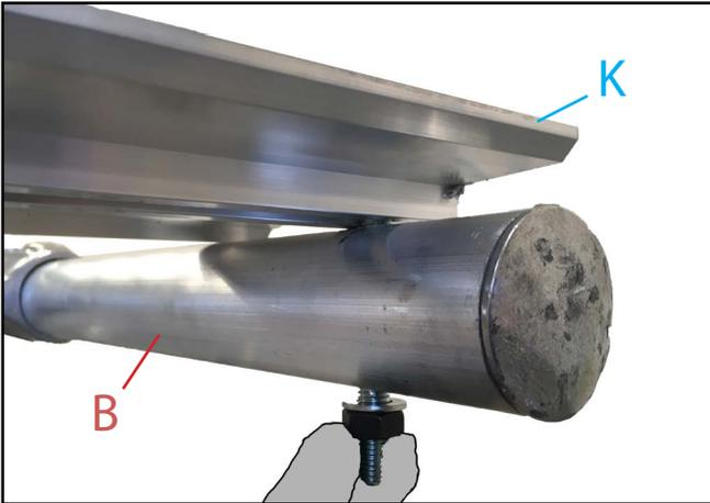
**12.** Add 1no. part (K) toe-board to part (B) uprights. Thread M10 x 80mm bolt through hole in upright and add nut and washer. Tighten to 15Nm.
