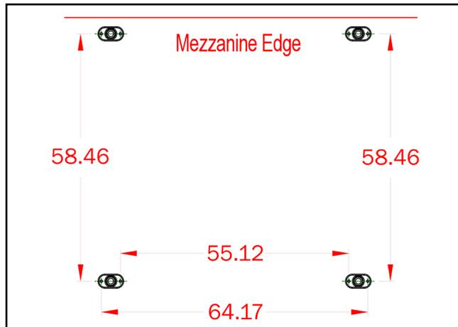
**1.** Using the above guide mark the position of the holes. Carefully drill a 12mm hole on each mark. Remove any debris using suitable extraction equipment.
