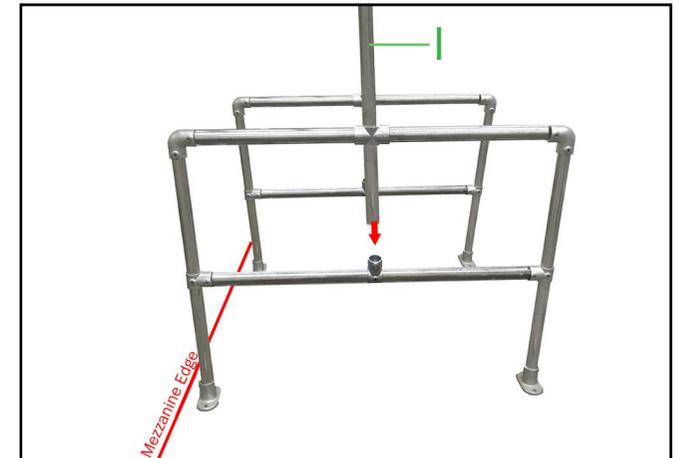
**5.** Slide part (I) upright rail through fittings on each frame. Tighten grub screws. Repeat for other frame.
