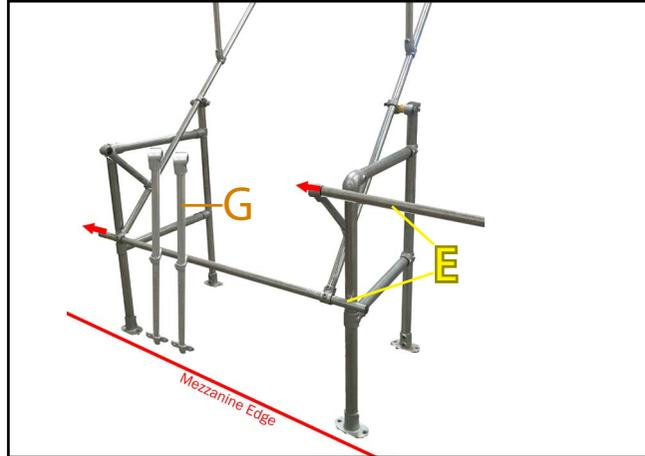
7. On Mezzanine leading edge slide 2no. part (E) horizontal tubes through the cantilever tube ends. During this process add 2no. part (G) vertical uprights with toe-board brackets onto horizontal tubes part (E).
