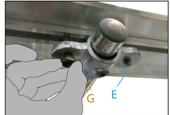
**8.** Mount toe-board (E) part to the (G) uprights by sliding 4No. bolt heads into the track along the back of the toe-board. Carefully align 2No. bolts so they fit through each of the M51-6 fitting. Add the washer and nut and loosely tighten to permit movement within the toe-board for adjustment in next step.
