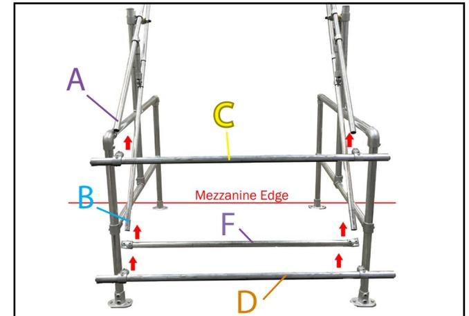
**11.** On opposite end to mezzanine edge mount horizontal tube part (C) to upper cantilever rails (A). Slide part (F) 5.9" up part (B) cantilever tubes and tighten using 1/4" hex key. Mount horizontal tube part (D) to lower cantilever rails (B). Tighten fittings using 1/4" hex key.
