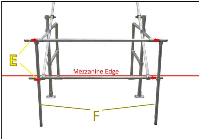
**9.** On opposite end to mezzanine edge slide 2no. part (E) horizontal through cantilever tube ends. Add 2no. (F) uprights onto ends of horizontal tubes. Tighten using 1/4" hex key.
