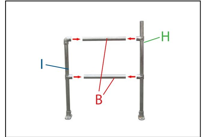
**2.** Build 2No frames using 1No. (H) upright, 1No. (I) upright and 2No. (B) horizontal parts per frame. Once tubes are fully inserted tighten grub screws using 5/16" hex key.
