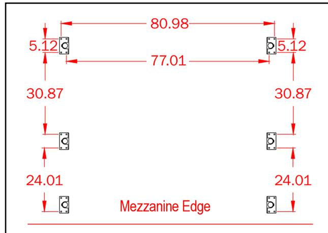
**1.** Lay components on safe flat working area. Using adequate fall protection device drill 12mm holes to allow feet to be attached using the above guide.
