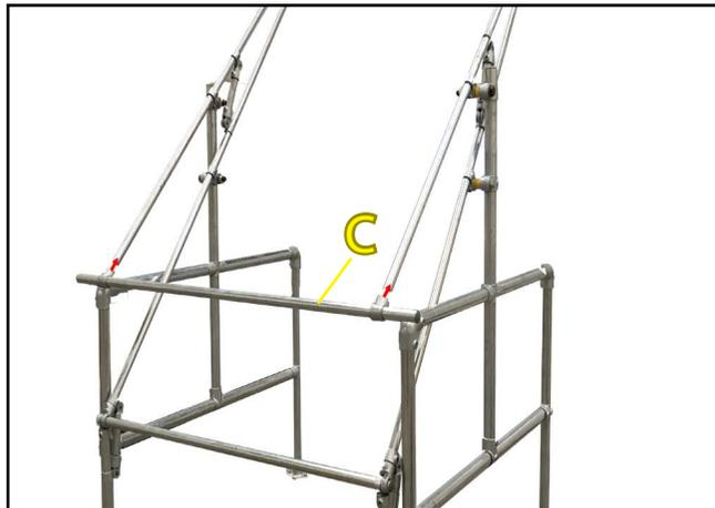
**10.** Add 1no. part (C) horizontal tube to mezzanine floor edge end as in diagram above. Tighten using 1/4" hex key.
