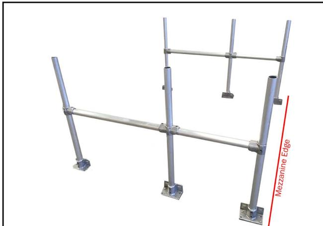
**3.** Align each frame to the pre-drilled holes. Slight adjustment of the fittings may be necessary to centre correctly with the holes. As per drawing, the frame uprights are off centre, so the centre post should be closer to the leading edge of the mezzanine.
