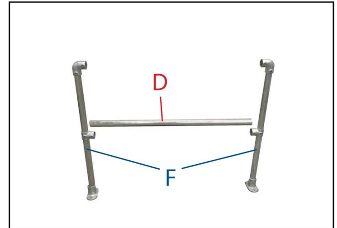
2. Build 2No frames using 2No. (F) uprights, 1No. (D) horizontal per frame. Once tubes are fully inserted tighten grub screws using 5/16" hex key.
