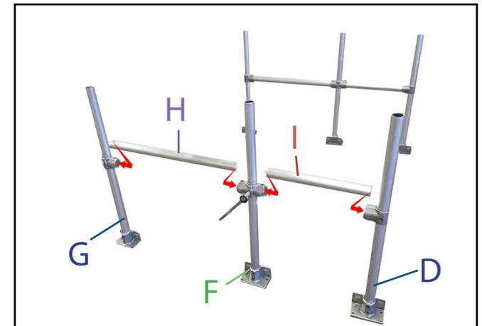
**2.** Build 2 frames using 1no. (D) part, 1no. (F), 1no. (G) per frame as above. Link upright posts using 1no. part (H) and 1 no. part (I) per frame and tighten grub screws using 5/16" hex key. Repeat process to make second frame.
