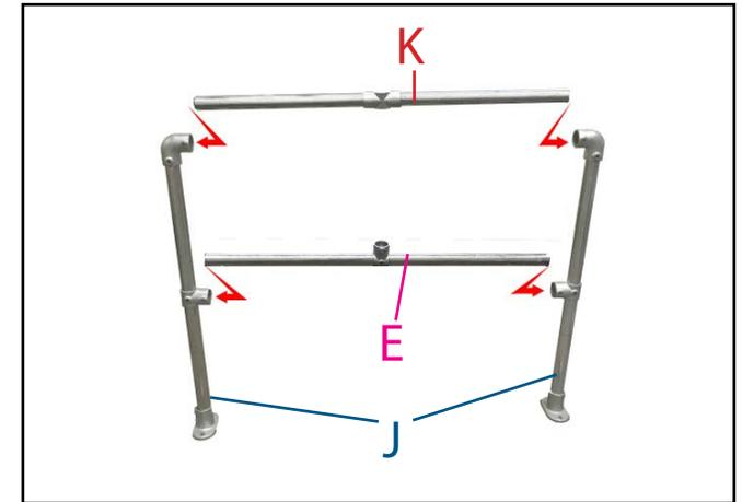
**2.** Build 2 frames using 2no. (J) uprights, 1no. (E) horizontal for the lower horizontal and 1no. (K) for the upper horizontal per frame. Once tube is fully inserted tighten grub screws using 5/16" hex key.
