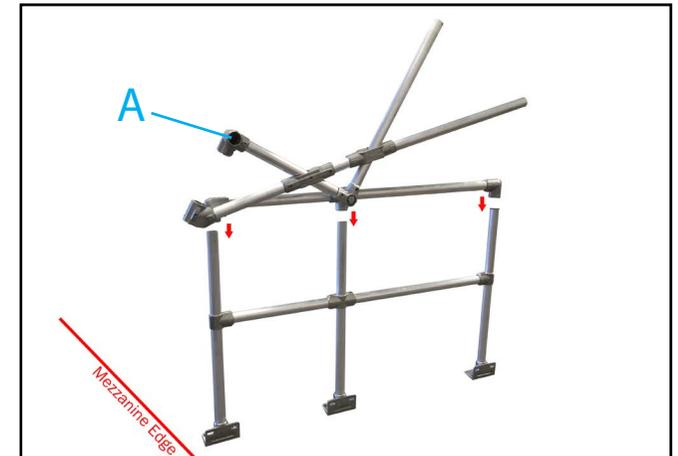
**5.** Add part (A) cantilever arms onto the frame, ensuring that the arm is positioned on the inside of pallet gate. Repeat for opposite frame.
