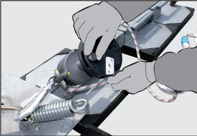
**V.** Pass the loose end of the Kernmantel Rope around the pig tail of the Rescue Hub. Hold the rope firmly in one hand. To take the load off the casualty, simply rotate and pull the Locking Pin upwards and rotate sufficiently so that the pin is disengaged from the Rescue Hub. Whilst holding the Kernmantel Rope you can move back towards the area where the casualty fell.
