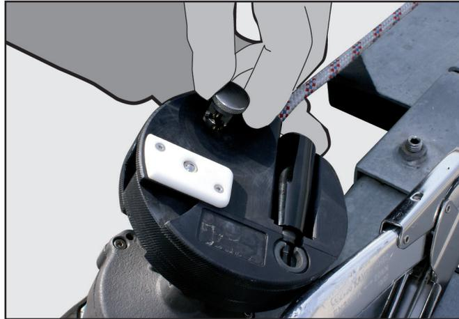
**m.** Once the Rescue Hub Kernmantel Rope is taught, rotate & lower the locking pin so that it engages with the body of the hub. When in place correctly, the hub cannot turn.
