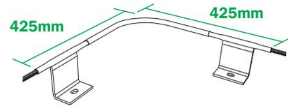
**CORNER TUBE - Wall mounted 90° - CNR-90-W**
