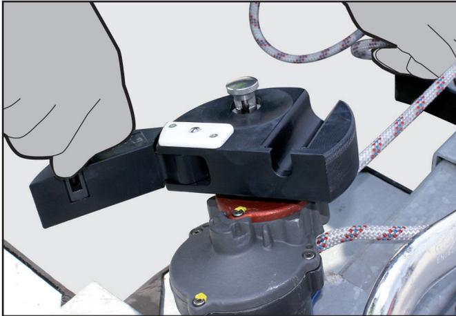
**r.** Start winding the Rescue Hub in a clockwise direction so that the Kernmantel Rope passes through the hub. If the rope does not move through the hub, pull on the free end of the rope. Continue to wind until the casualty's primary rope becomes slack.
