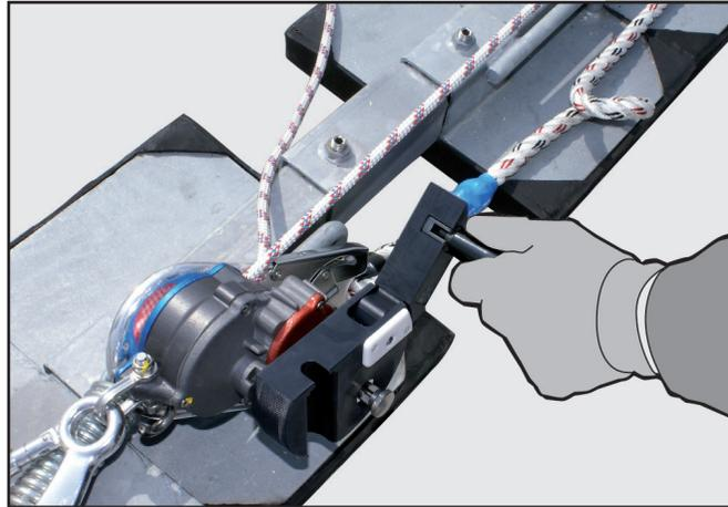
**s.** Once the casualty's primary rope is slack enough to detach their primary hook/karabiner from the anchorage point, stop winding and engage the locking pin by lifting, rotating & then lowering it. Ensure the pin is engaged against the body of the Rescue Hub. When in place correctly the Hub cannot turn.
