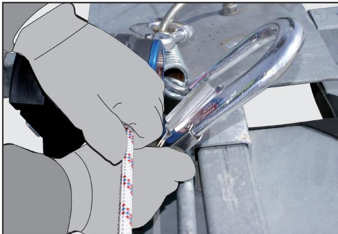
**t.** You can now remove the casualty's slack primary rope from the anchorage point as shown above.
