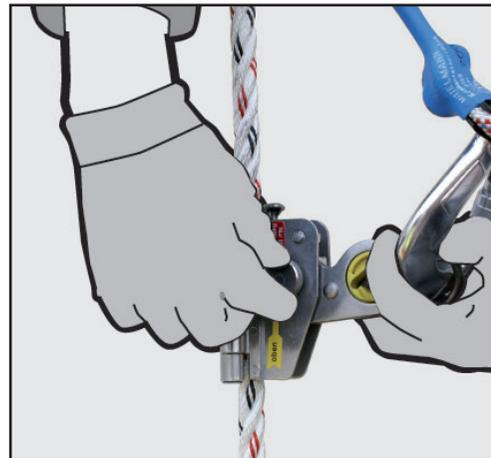
**j.** Once the Rescue Rope Grab is closed ensure the Screw Gate is then tightened into position.
