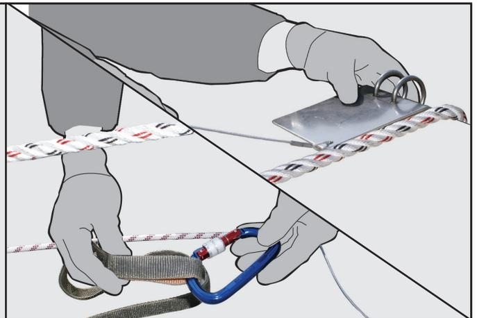
**d.** Ensure the Edge Protector is connected to the anchorage point, this may need to be extended in some cases via a webbing or rope sling. Place the Edge Protector over the edge ready for the rescue operation.
