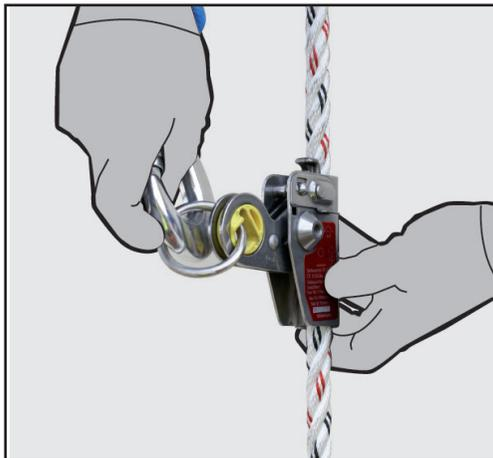
**i.** (cont) Ensure the casualty’s rope is correctly positioned inside the Rescue Rope Grab. Close the Rescue Rope Grab.
