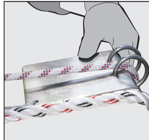
**k.** Position the Rescue Kernmantel Rope over the Edge Protector. Now carefully lower the Rescue Rope Grab down towards the casualty. The Rescue Rope Grab device will descend easily under gravity to the “D” ring of the casualty’s harness.
