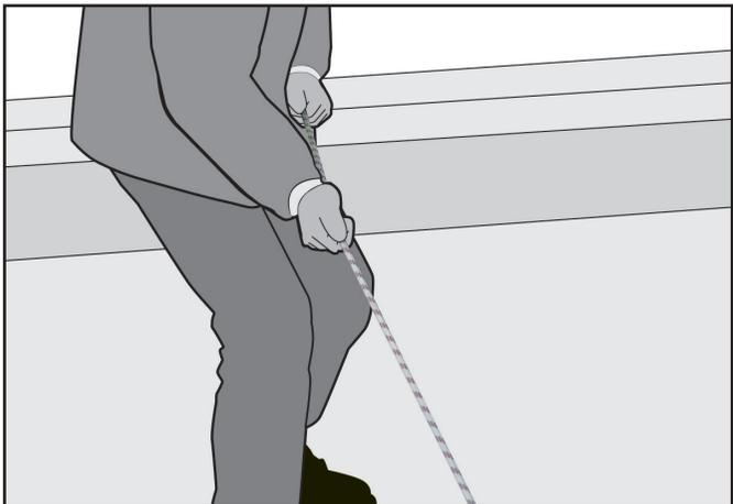
**c.** Start walking towards the area where the casualty has fallen whilst still holding the Rescue Rope Grab. When you reach this area, kneel down and continue to pull out sufficient rope to reach the “D” ring on the casualty’s harness.
