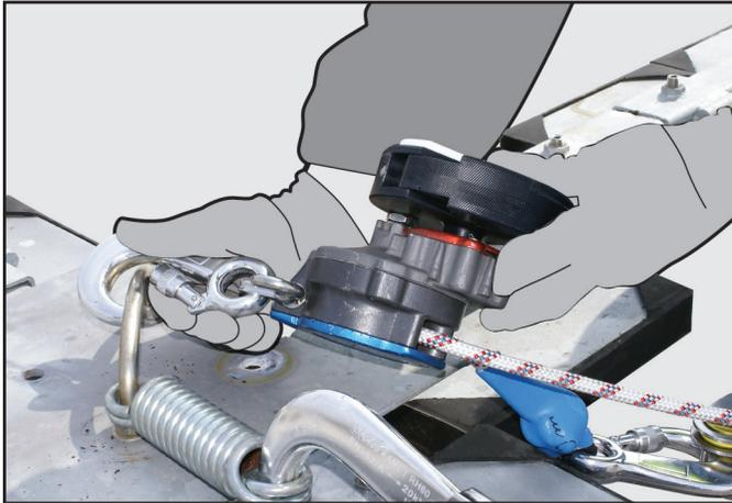
**a.** Connecting to the same or an alternative suitable anchorage point. Connect the Rescue Hub device using the Screw Gate Karabiner fitted directly to the Rescue Hub. Ensure the Screw Gate is tightened once connected to the anchorage point.
