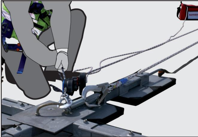
**l.** Return to the anchorage point where the Rescue Hub is connected. Pull any excess Kernmantel Rope through the Rescue Hub by pulling the free end of the rope which is stored in the bag.
