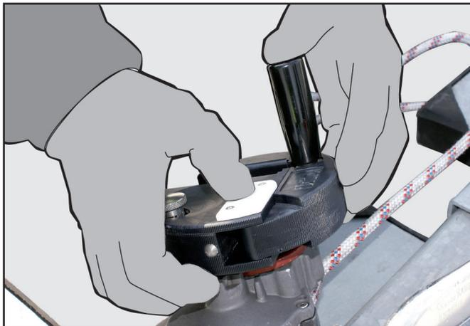
**o.** With the black handle in position push the silver ball bearing positioned in the centre of the white plate as shown above.
