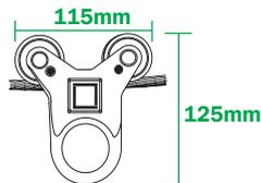
**OVERHEAD WHEELED TRAVELLER - KOTRAV**
