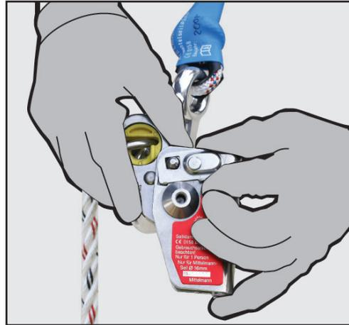
**f.** Turn the Rescue Rope Grab over and push the lever in an upwards direction.
