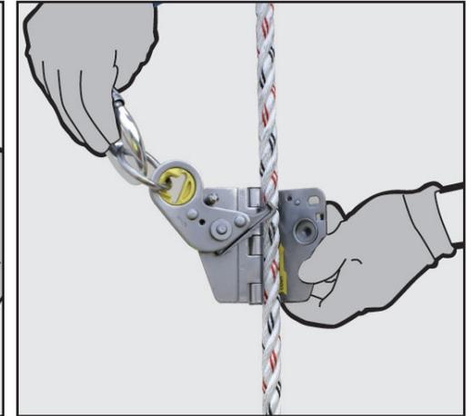
**h.** Ensure you have adopted a “fall restraint” position. Carefully lean over the leading edge and pass the open Rescue Rope Grab (with the arrow in the up direction) around the back of the casualty’s rope. (cont)
