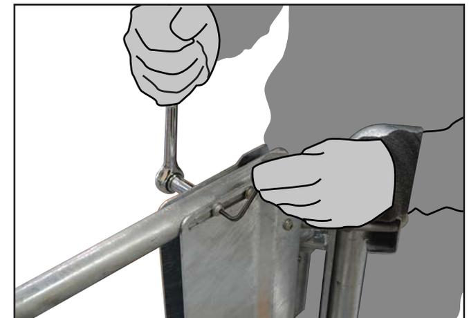
**E.** To extend the gates width to the required opening simply loosen the hex nuts and bolts on the top guardrail using a 3/16" Allen Key and 1/2" socket.
