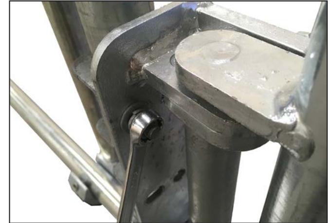
**B.** Using a 11/16" or 1/2" flat washer and nut connect the U bolt to the Support Leg/Structure and tighten.
